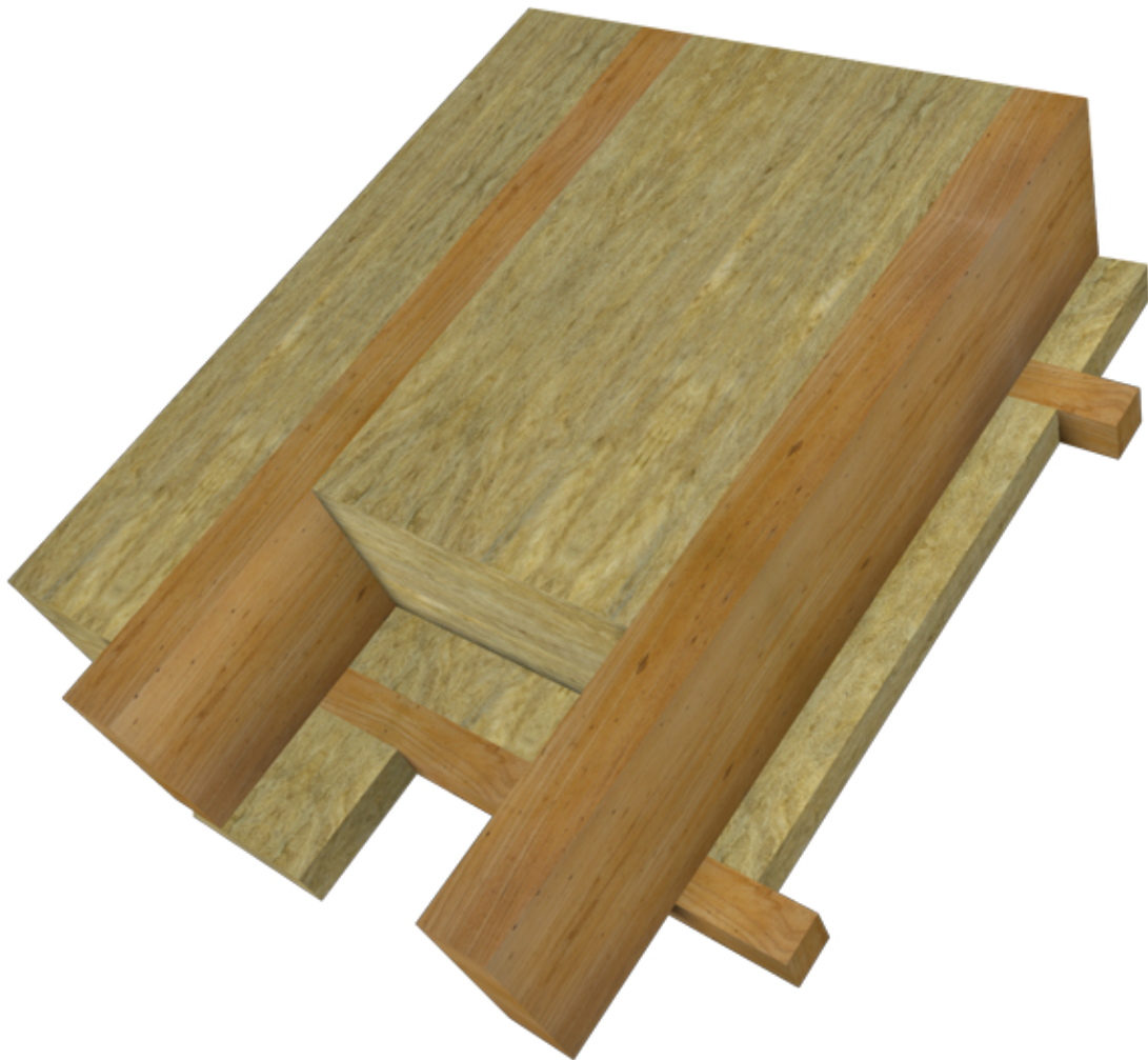
Figure 3: Thermal bridging running in two different directions
